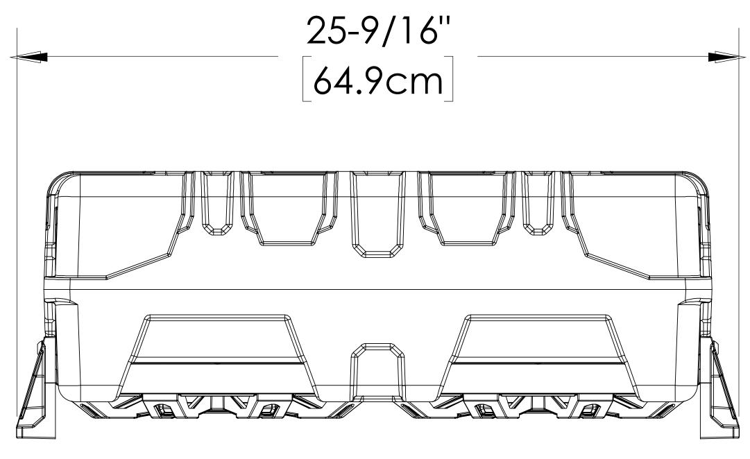
Enclosure dimensions listed in down-firing configuration
